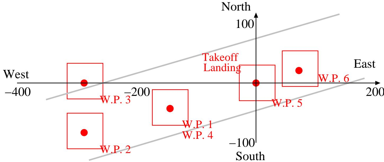
The UAV was required to fly over the 60-meter square zone of each waypoint, and to fly at an altitude of 15 meter.
