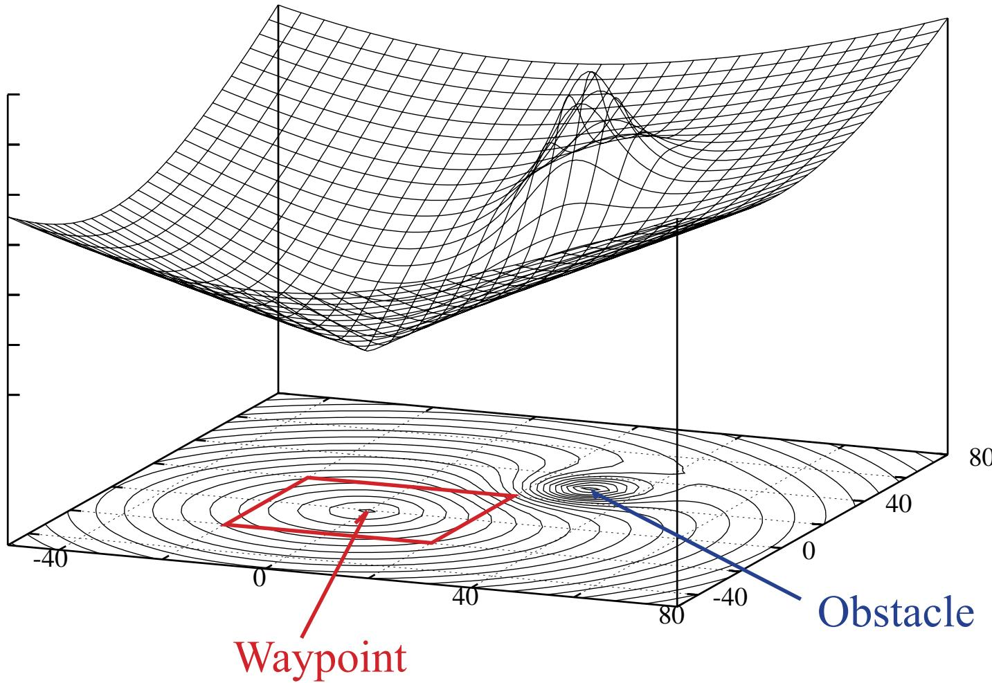
The desired heading angle,  $\psi_d$ , is determined by the gradient of the artificial potential field.
